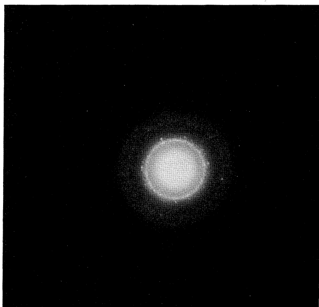
Fig. 4. Selected area electron diffraction pattern of the colloidal copper dispersion obtained by reducing copper(II) sulfate with sodium tetrahydroborate in the presence of dextrin; [\text{CuSO}_4]_0 = 5.0 \times 10^{-3} , [\text{NaBH}_4]_0 = 1.0 \times 10^{-2} , and [\text{monomeric residue of dextrin}]_0 = 2.0 \times 10^{-1} \text{ mol dm}^{-3} .
